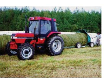
The tube-o-later system is an automated version of the home-made system. Specialized equipment uses guides to raise the bales so they can be moved through the hoop and into the plastic tube folded around it. The hoop starts at the end of a row of bales and moves forward as bales are inserted, leaving a long and sealed tube of silage behind.
