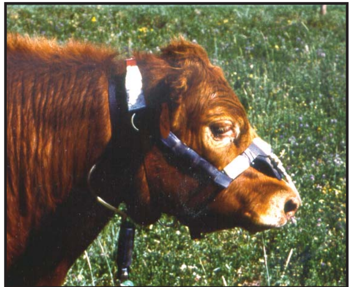
Figure 2. Apparatus for Collecting Methane Gas
